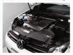
the performance features guaranteed by BMC filter technology. The CRF air box is powered by a dynamic intake and is very efficient. Its special shape ensures it can provide a significant increase in the air intake to the engine and a drastic reduction of its temperature.
